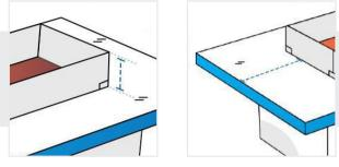
8. Distance From Top Box Depth To Counter Edge: Distance From Top Box Depth To Counter Edge of the Rectangular Fire Pit
